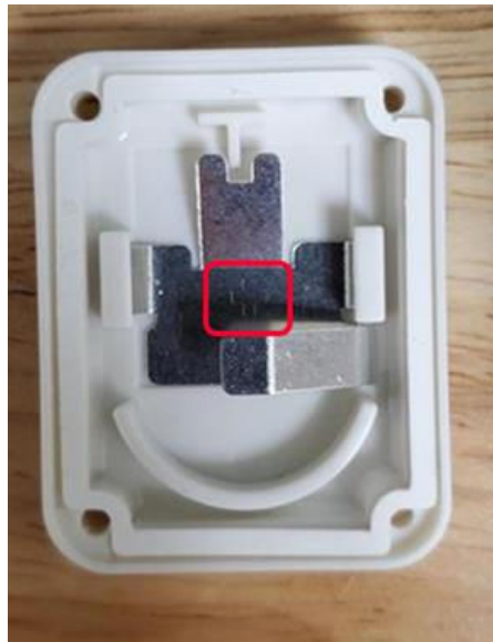
Figure 2-10: Proper Gasket Appearance
