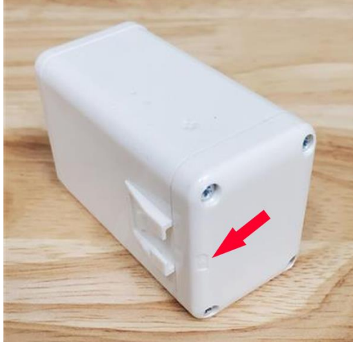
Figure 2-11: Proper Replacement Orientation of the Battery Cover
