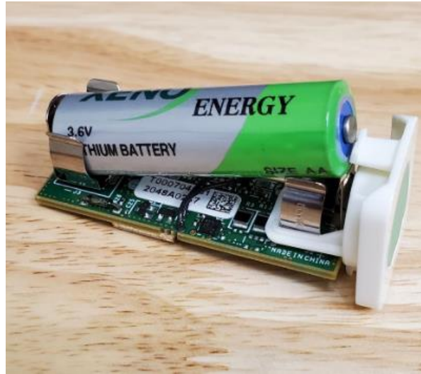
Figure 2-6: Battery Polarity Orientation
